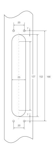
Drilling and hole dimensions.
