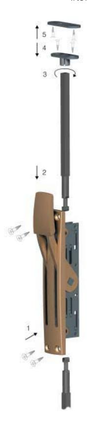
Quick-bolt 3000 fitting diagram.
