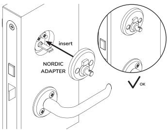
Mount the adapter with two screws using a Philips screwdriver.
